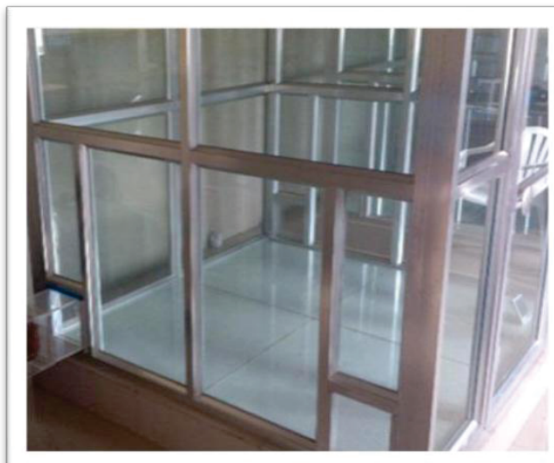
Peet – Grady Chamber for Insecticide testing
