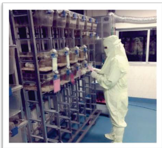
Individual Ventilated Caging System
