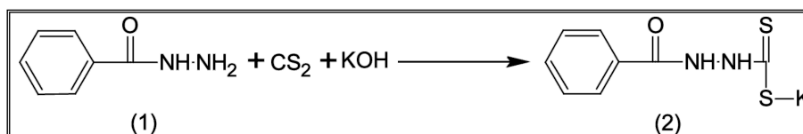
Fig. 25: Preparation of potassium salt of 2-benzylidithio carbazinic acid
