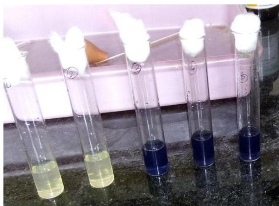
Figure 1: Colorimetric analysis of Vit C. From left to right Tube no. 1:10 mg; tube no. 2:1mg; tube no. 3:0.1 mg, tube no. 4:0.01 mg; tube no. 5 0.001mg.
